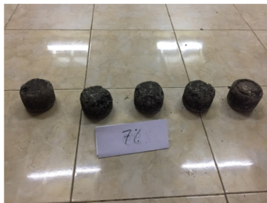
Figure 4. Morphology of specimens after abrasion loss test
