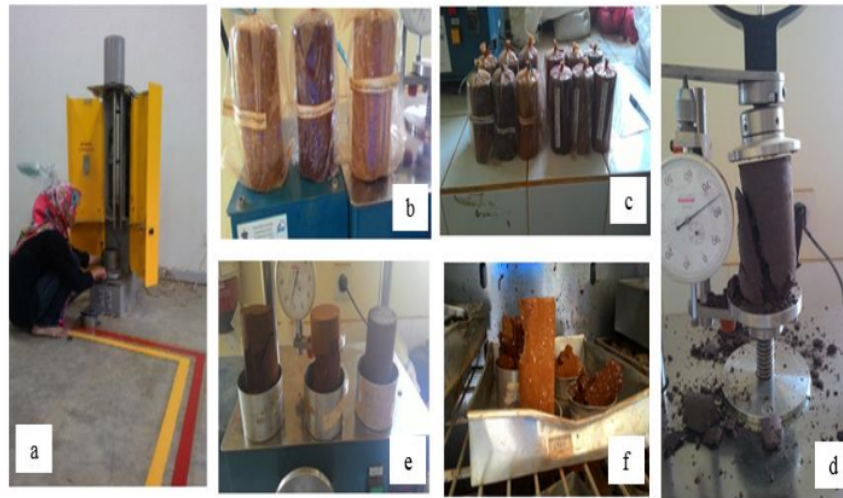
Figure 2. Unconfined compression strength testing procedure: a) compaction test, b) cylindrical untreated and treated soil sample, c) curing process, d) unconfined compression test (UCT), e) sample weighing after testing, f) drying in an oven.
