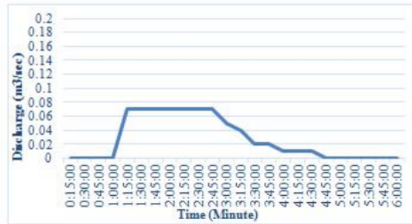
Figure 8. FEB Outfall Flood Hydrograph
