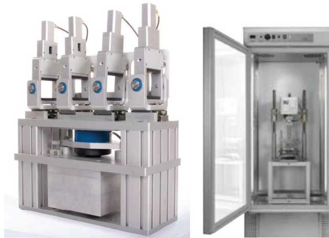
Gambar 4. Alat uji four point bending beam machine
