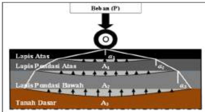
**Gambar 2.1:** Distribusi Beban Roda Pada Perkerasan (Wiryanto, 2011)
