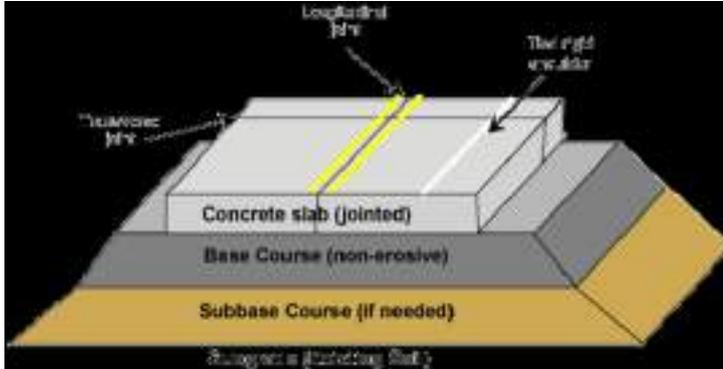
**Gambar 1.3:** Konstruksi perkerasan kaku (Rigid Pavement) (Sugiyanto, 2019)
